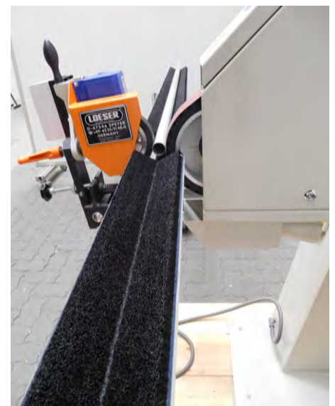
Guide trough with brush support for workpiece protection
