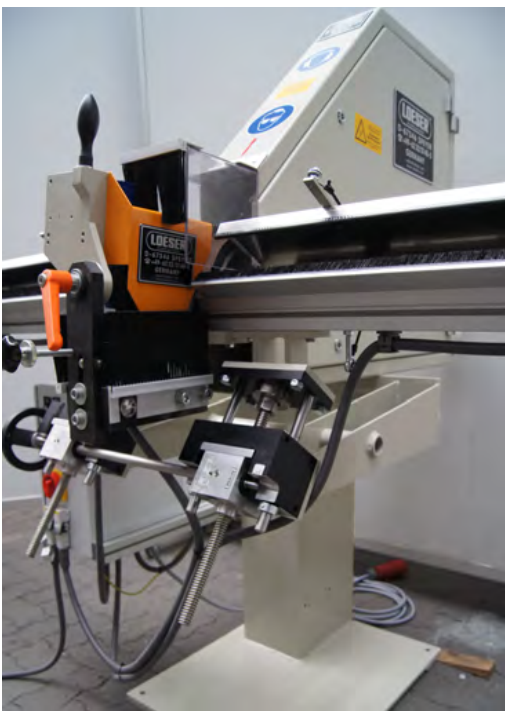
Central height adjustment with two spindles and lateral support for heavy parts
