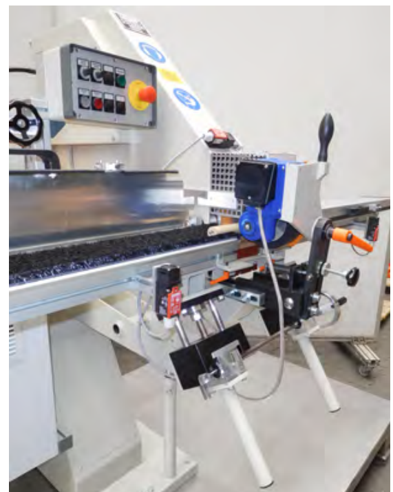
Safety cover of the guide rail with electrical lock
