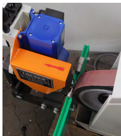
Guide trough with brush support for workpiece protection
