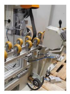
Pneumatically supported contact wheel & BA
