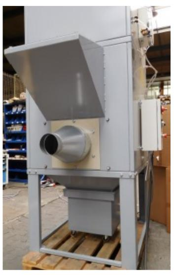
Pressure relief flap of the extraction for aluminium dust
