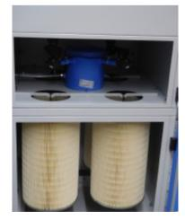
Cartridge filter with compressed air pulse cleaning
