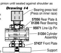
4. Invert rotor pinion in support. Install 56047 Rotor Key and 57113 Blade and Rotor Set onto
